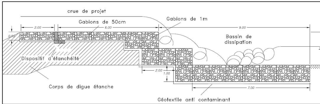
Figure 10: Cross section of the stepped gabion spillway
