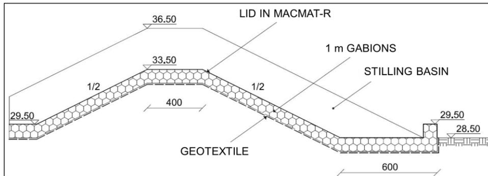
Figure 7: cross section of the gabion spillway
