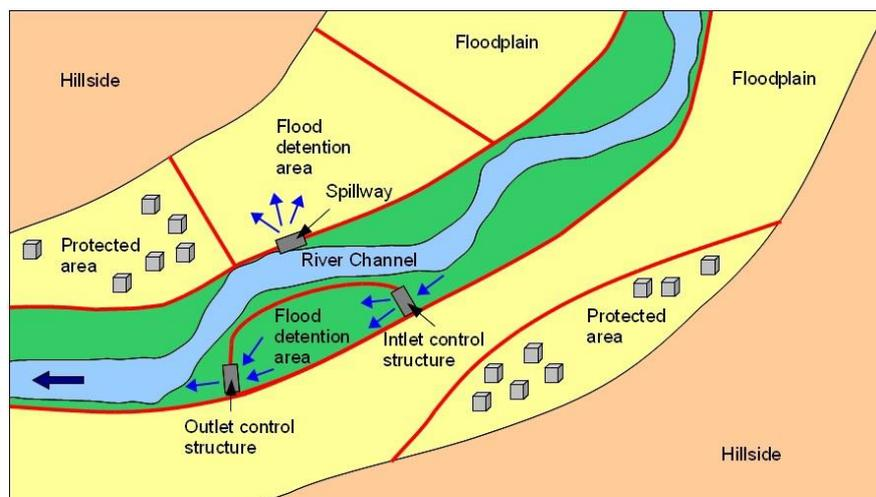
Figure 1 Flood retention scheme [1]
