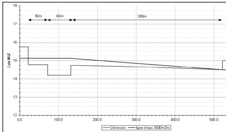
Figure 9: Longitudinal profile of the Lunel spillway for Q=3000 m<sup>3</sup>/s
