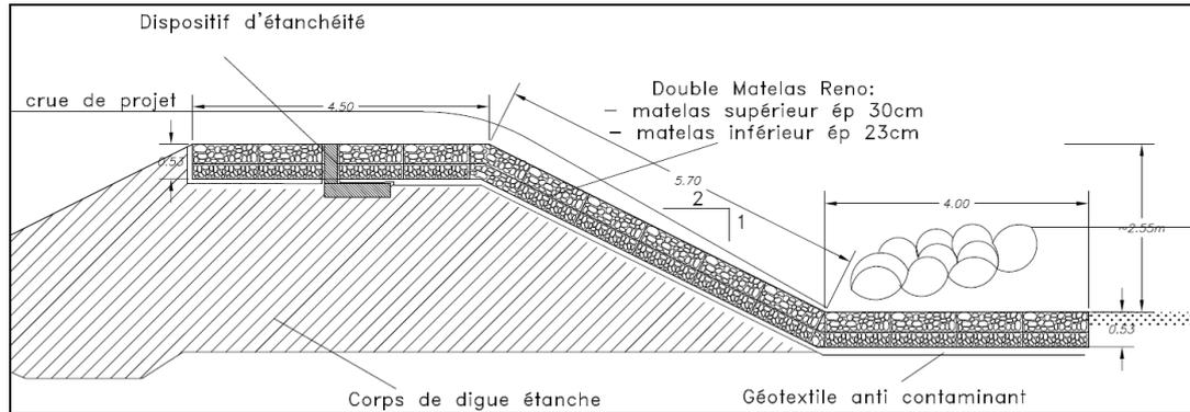
Figure 11: Cross section of the inclined Reno mattress spillway
